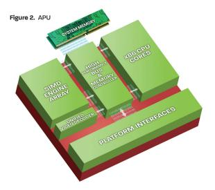
Until now, transistor budget constraints typically mandated a two chip solution for such systems, forcing system architects to use a chip-to-chip crossing between the memory controller and either the CPU or GPU as shown in Figure 3. These transfers affect memory latency, consume system power and thus impact battery life. The APU's scalar x86 cores and SIMD engines share a common path to system memory to help avoid these constraints.
